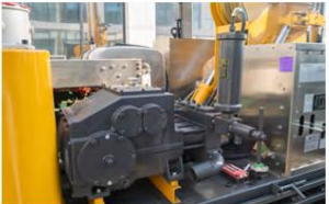
泥浆泵 Mud pump
