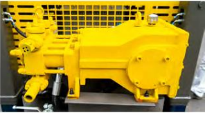
泥浆泵 Mud Pump
